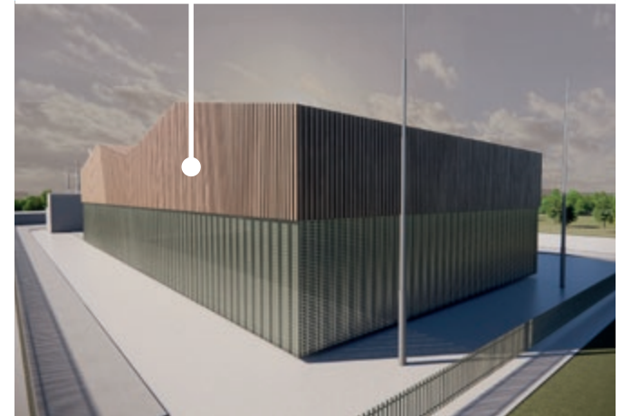
Upper-level transitions into plasticised timber cladding
